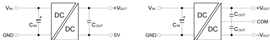
Figure 1: Typical Application circuit
